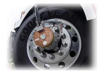
In the past, strain was often measured statically in a laboratory at very slow rotational speeds, and repeated tests were required to gather all the necessary data. A complete static test could take more than an hour to complete. Now, with digital telemetry, a dynamic test can be run and all the data gathered in less than a minute.
